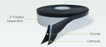
A Rolled-Ribbon roll consists of long, narrow cathode and anode strips – "ribbons" – that are tucked into separate folds of a long length of separator folded into a Z-shape and together spiral wound.
